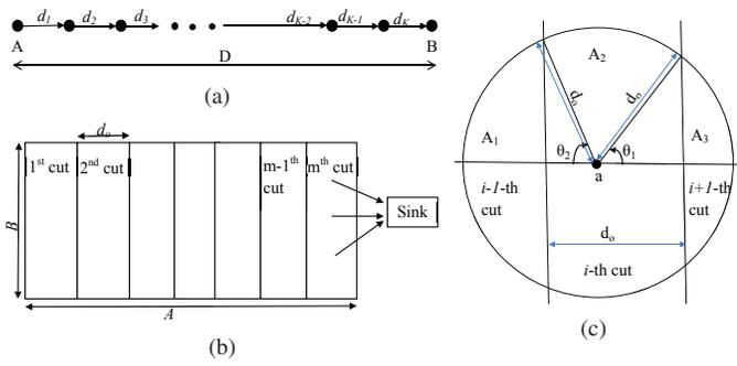
Fig. 2. (a) Introducing  $K - 1$  relay between A and B, (b) A sensor network with  $N$  nodes in a field of  $A \times B$ , (c) Calculating overhearing at the  $i$ -th cut.
