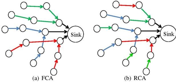
Fig. 1. Proposed data collection trees with multiple channels. Each color represents a different channel.
