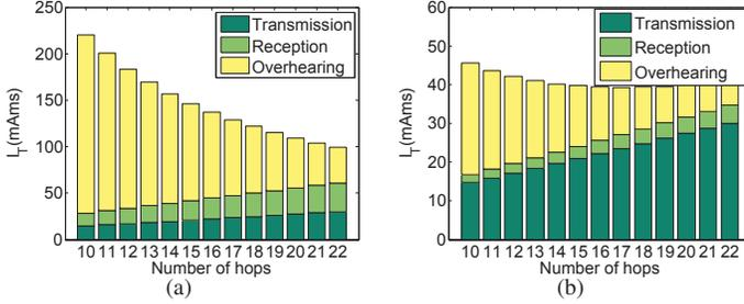
Fig. 3. Variation of  $I_T$  with  $K$  when  $D = 200$  meters and  $\rho = 0.0125$  nodes/meters<sup>2</sup> for MICA2 motes (a) with typical value of  $I_r = 10$  mA, and (b) with a fictitious value of  $I_r = 1.5$  mA.
