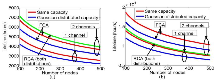
Fig. 6. Expected network lifetime with different number of nodes (a)  $\alpha_r = 10$  mA and (b)  $\alpha_r = 1.5$  mA
