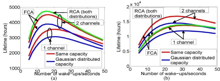
Fig. 7. Expected network lifetime with different wake-up rates (a)  $\alpha_r = 10$  mA and (b)  $\alpha_r = 1.5$  mA
