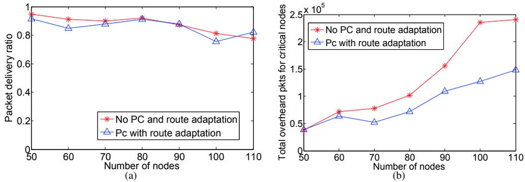
Fig. 5. Comparison of (a) packet delivery ratio and (b) packets overheard by the critical nodes with different node density.
