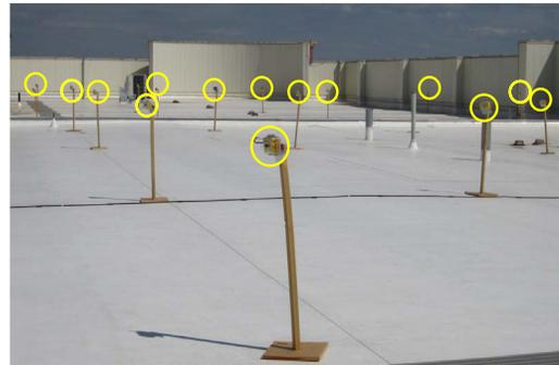
Fig. 6. A 25-node wireless sensor network testbed.
