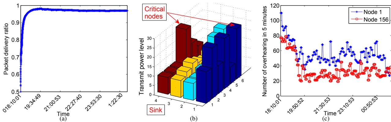
Fig. 7. (a) Overall packet delivery ratio to the sink over time. (b) Transmit power levels of different nodes, power level 27 corresponds to -1 dBm and power level 9 corresponds to -13.4 dBm. (c) Number of packets overheard by the two critical nodes over time.
