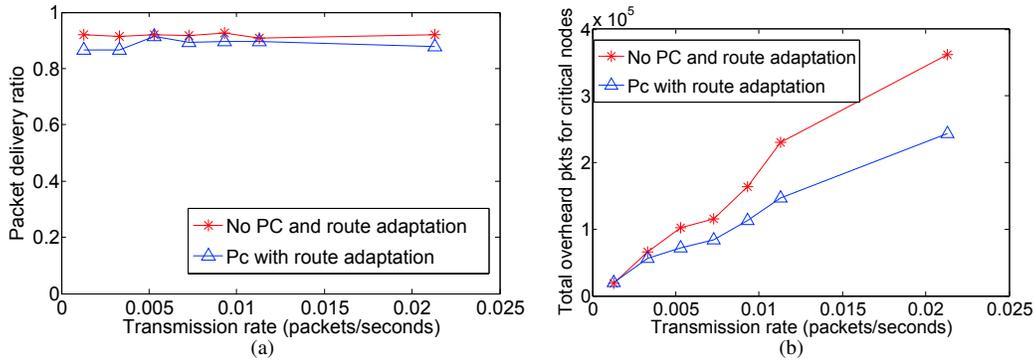
Fig. 4. Comparison of (a) packet delivery ratio and (b) packets overheard by the critical nodes with different rates.
