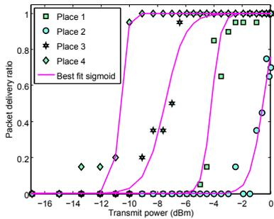
Fig. 2. Sigmoid best fit curve of delivery ratio vs transmit power.
