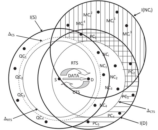
Fig. 2. Effect of interferers in presence of RTS/CTS for test link  $S \rightarrow D$
