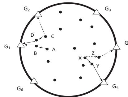
Fig. 1. Wireless mesh network architecture with multiple gateways
