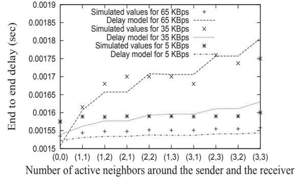
Fig. 3. Variation of delay with different number of active neighbors of sender and receiver. The terms in x axis are  $(n_a, n_b)$ .
