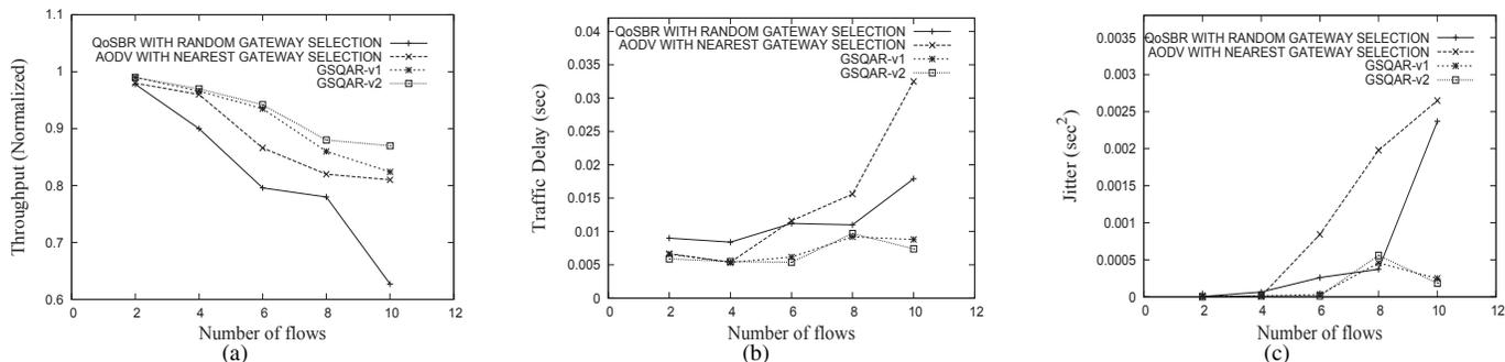
Fig. 4. Comparison of (a) Throughput (b) Delay (c) Jitter
