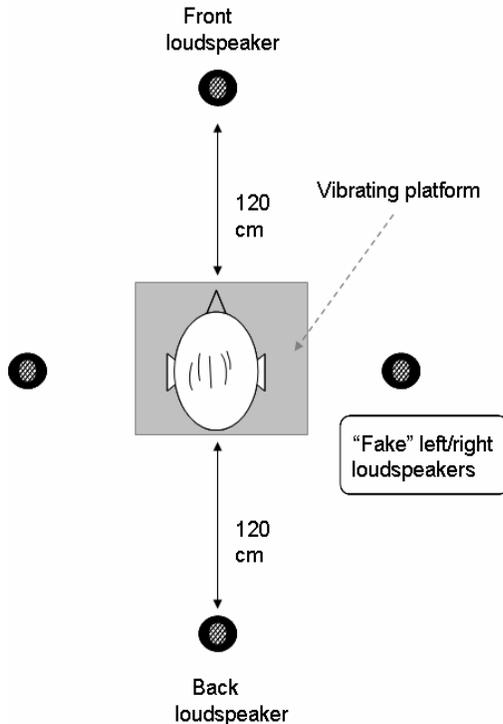
Figure 1 Top-view of the experimental setup
