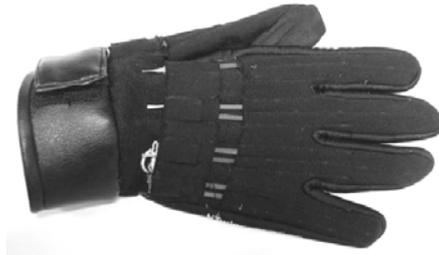
**Figure 1: The Percro data-glove.**
