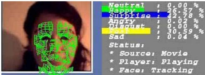
**Figure 3** – Example of our real-time working system with the emotional state probabilities displayed on the right.
