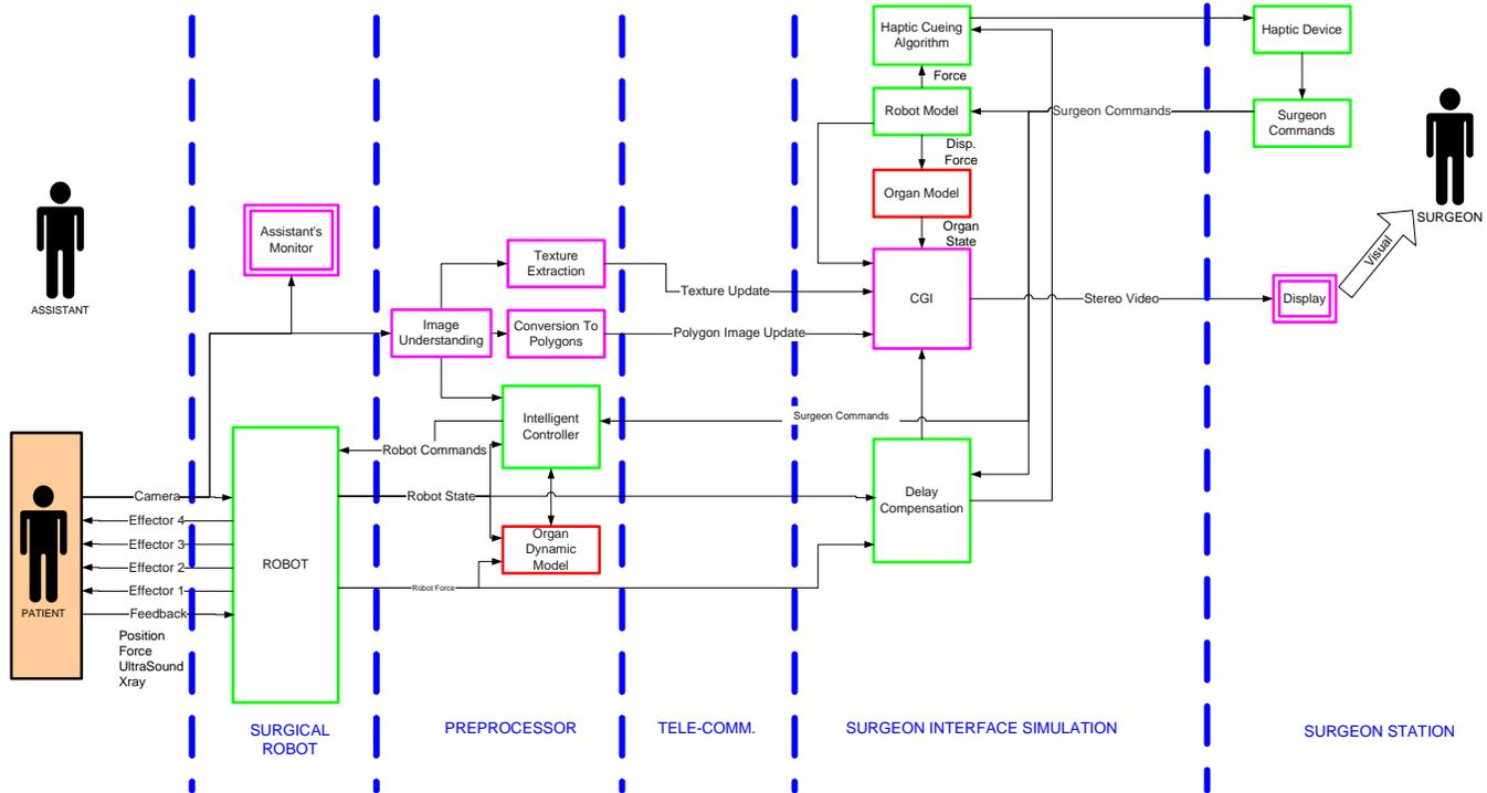
Figure 6 Block diagram of the surgical telerobotics system
