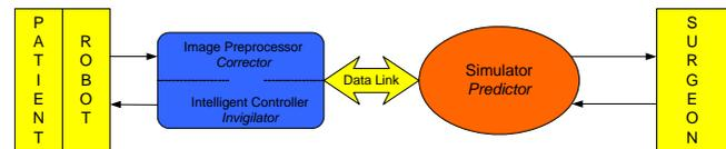
Figure 8 Surgical telerobotics as a tele-presence system
