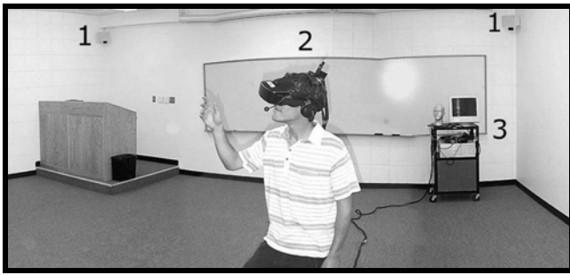
Figure 1: A depiction of the immersive virtual environment system. The components are 1) WorldViz PPT position tracking cameras, 2) Virtual Research V8 head-mounted display and Intersense orientation tracking sensor, and 3) image generator.
