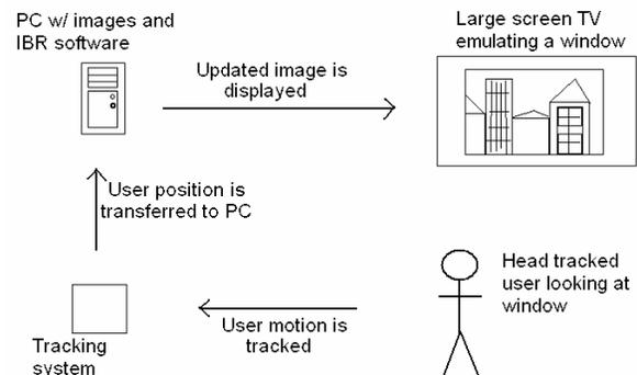
**Figure 2: Schematic overview of the system.**
