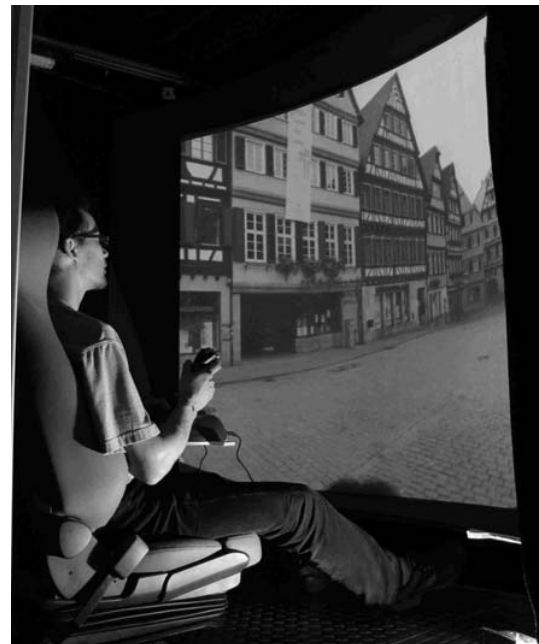
Figure 3: Participant seated in front of curved projection screen displaying a view of the Tübingen market place. The simulated FOV matched the physical FOV of 54°x40.5°.
