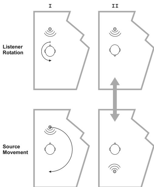
**Figure 1 Physical comparison of Listener Rotation (LR) and Source Movement (SM). Unless the surfaces are perfectly absorbing and source / listener are located as shown in the left panels, the impulse responses in the listening position will be different for LR and SM.**
