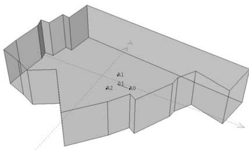
**Figure 3 The acoustic model used in the experiment: A model of the market place in Tübingen, Germany. A0, A1, A2 denotes source positions and O1 denotes the receiver position.**
