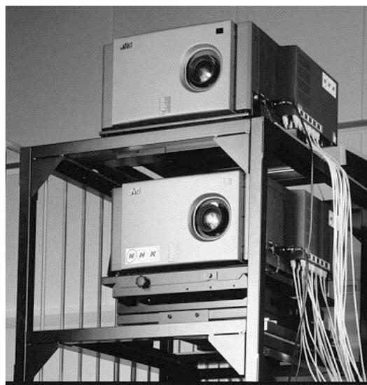
Figure 2. Dual green projection unit (lower) and red/blue projection unit (upper).
