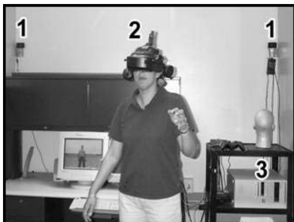
Figure 1. A depiction of our virtual environment system: 1) position tracking cameras; 2) HMD and orientation tracking sensor; 3) image generator.
