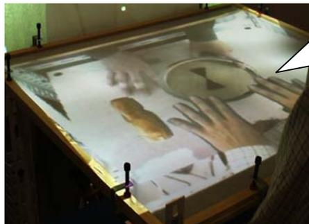
Projecting a synthesized video image of local and remote tabletop onto a screen over the table
