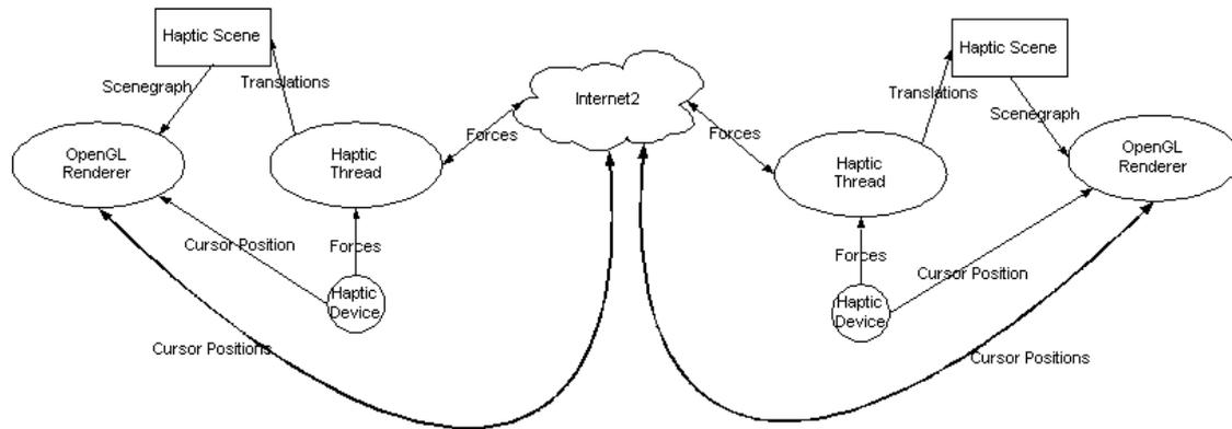
Figure 5: Software Architecture
